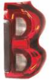
Tail Lamp Unit Lower LED Red Lens Scorpio S11
